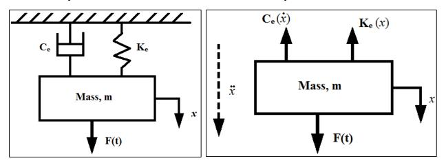
The analytical model, seen above to the left, will represent the cutting mechanical operation. Where, F(t),  $K_{e}$ , and  $C_{e}$ , denote the given applied force, equivalent spring constant, and damping coefficient respectively. Using the analytical model, a free-body diagram (F.B.D) is developed, seen above to the right. For both diagrams x,  $\dot{x}$ , and  $\ddot{x}$  denote the positive direction of the system's displacement, velocity, and acceleration.
